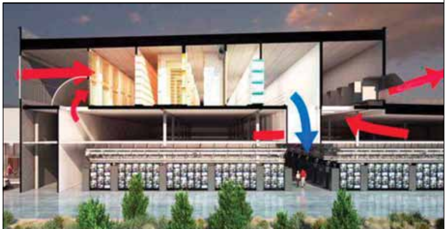
Figure 2. Rendering of airflow through the OCP datacenter.
